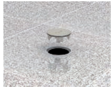
Mounting of tube body Insert the tube body cover into the tube body seat and lower it. Unlock the tube body by turning it to the right and close it flush to the floor.
