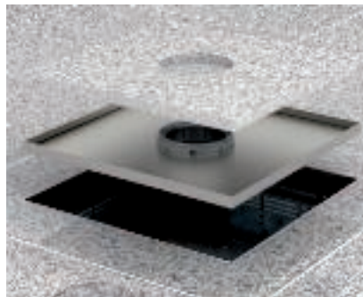
Laying the floor covering in the RKF cassette Lay the floor covering in the cassette and stick it down. Seal the remaining gap between the floor covering and the cassette with suitable materials.
