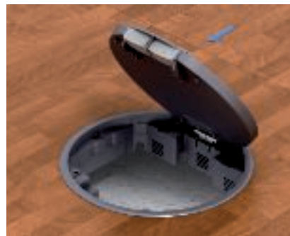
Closing of the hinged lid for GESR round service outlet Close the lid. Press on the lid above the lid hinge until the end position is reached.
