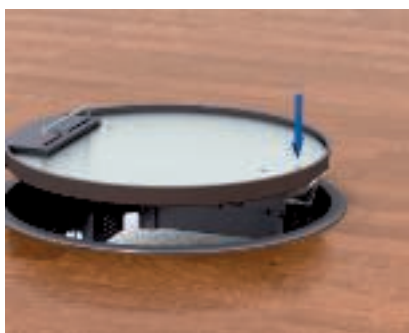
Installation of the hinged lid for GESR round service outlet Insert the lid hinge in the bracket. Close the lid. Press on the lid above the lid hinge until the end position is reached.
