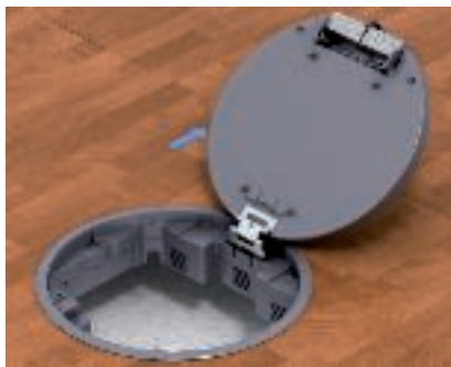
Opening of the hinged lid for GESR round service outlet and depositing inwards Push the hinged lid through an angle of 90° (stop). The hinge locks on the carpet protection frame.
